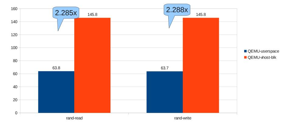
IOPS (K) fio test on 8 ramdisk based device with 4KB rand read and wrtie
