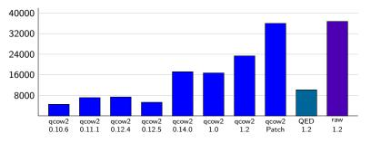
Write throughput in kB/s during sequential cluster allocation; 256k blocks; cache=none (iozone)
