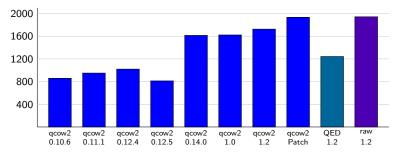
Write throughput in kB/s during sequential cluster allocation; 8k blocks; cache=none (iozone)
