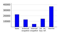
Write throughput in kB/s during sequential cluster allocation; 256k blocks; cache=none (iozone)
