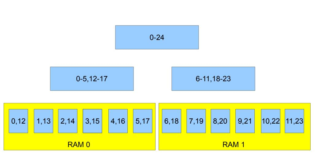
Example of a common 2 nodes, 2 sockets, 12 cores, 24 threads system
