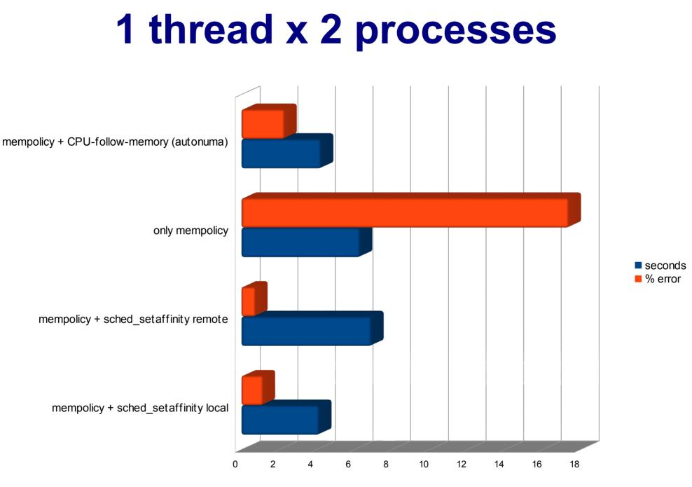
Only 2 CPUs used, 2 nodes 2 sockets 12 cores 24 threads
