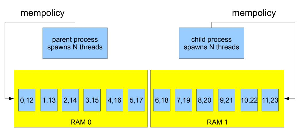
The host CPU scheduler understand the parent process has most of the RAM allocated in NODE 0 and the child in NODE 1 No scheduler hints from userland Mempolicy() doesn't have any scheduler effect
